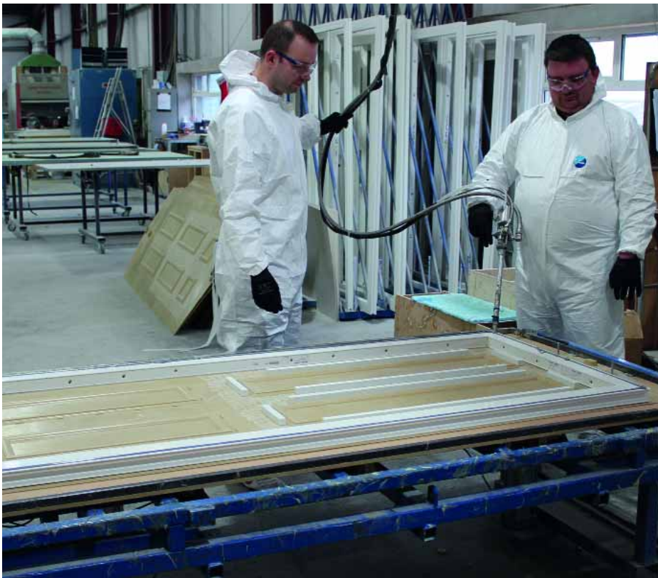
Crestabond structural adhesive bonding being applied to a New World door
